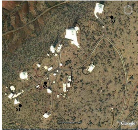
Figura 3. Aerial view of El Teide observatory taken from Google–Earth. Black circles labeled as S1, S2 and S3 correspond to the locations where seismic noise measurements were carried out.
